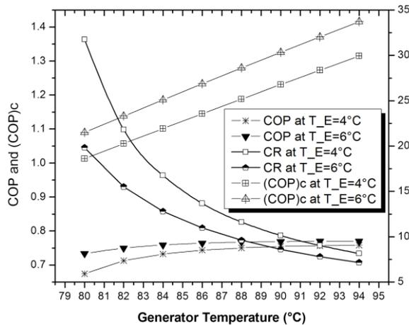
Fig-5: Variation of COP and COP<sub>c</sub> at different evaporator temperatures when the generator temperature is varied [T<sub>C</sub>=35°C, T<sub>A</sub>=40°C, Q<sub>E</sub> = 10 kW, ε<sub>1</sub> = 70%, ε<sub>2</sub> = 70%, η<sub>p</sub> = 95%]
