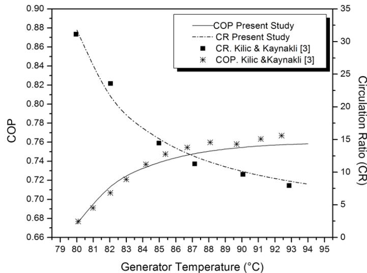
Fig-2: Comparison of COP and CR values with Kilic and Kaynakli [ $T_E = 4^\circ\text{C}$ ,  $T_C = 35^\circ\text{C}$ ,  $T_A = 40^\circ\text{C}$ ,  $\epsilon_1 = 70\%$ ,  $\epsilon_2 = 70\%$ ,  $\eta_p = 95\%$ ]
