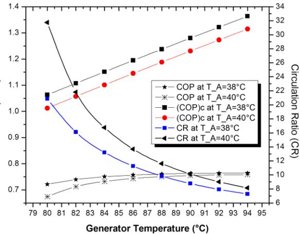
Fig-6: Variation of COP and COP<sub>c</sub> at different absorber temperatures when generator temperature is varied [T<sub>C</sub>=35°C, T<sub>E</sub>=4°C, Q<sub>E</sub> = 10 kW, ε<sub>1</sub> = 70%, ε<sub>2</sub> = 70%, η<sub>p</sub> = 95%]
