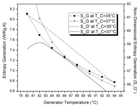
Fig-9: Entropy generation & non-dimensional entropy generation at different condenser temperatures for varying generator temperature [T<sub>A</sub> = 40°C, T<sub>E</sub> = 4°C, Q<sub>E</sub> = 10kW, ε<sub>1</sub> = 70%, ε<sub>2</sub>=70%, η<sub>p</sub> =95%].
