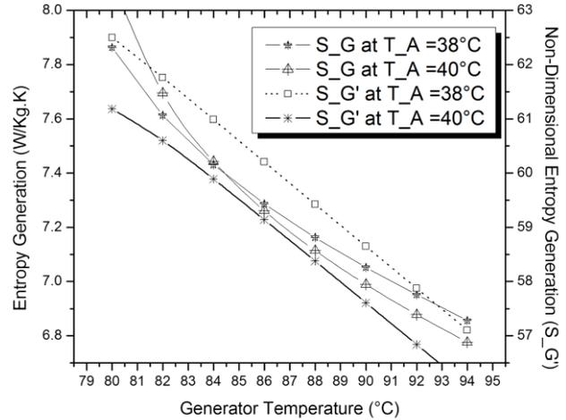
Fig-8: Entropy generation & non-dimensional entropy generation at different absorber temperatures for varying generator temperature [T<sub>C</sub> = 35°C, T<sub>E</sub> = 4°C, Q<sub>E</sub> = 10kW, ε<sub>1</sub>=70%, ε<sub>2</sub>=70%, η<sub>p</sub> =95%]
