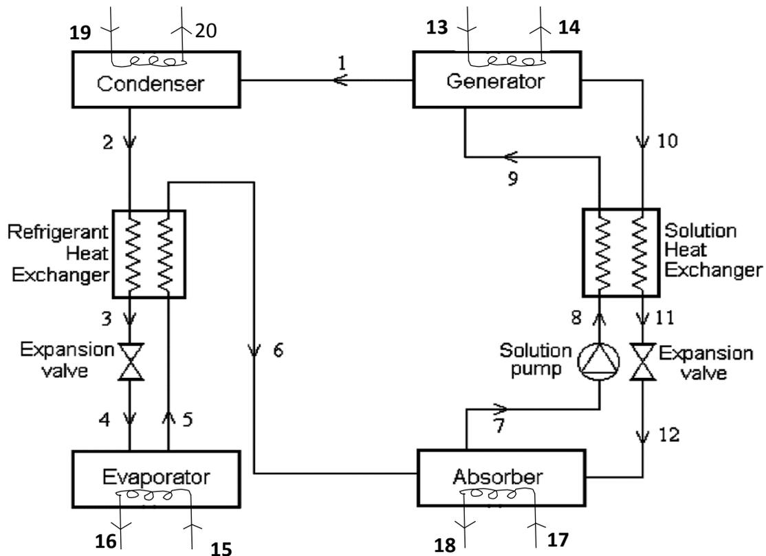
Fig-1: Block diagram of a vapour absorption refrigeration cycle
