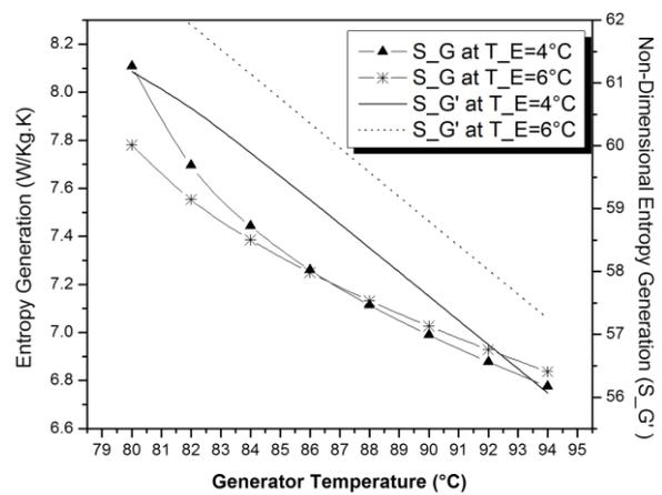
Fig-10: Entropy generation & non-dimensional entropy generation at different evaporator temperatures for varying generator temperature [T<sub>C</sub> = 35°C, T<sub>A</sub> = 40°C, Q<sub>E</sub> = 10 kW, ε<sub>1</sub> = 70%, ε<sub>2</sub> = 70%, η<sub>p</sub> =95%].
