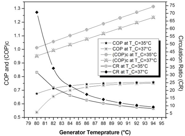
Fig-4: Variation of COP, COP<sub>c</sub> and CR at different condenser temperatures when generator temperature is varied. [T<sub>E</sub> = 4°C, T<sub>A</sub> = 40°C, Q<sub>E</sub> = 10 kW, ε<sub>1</sub> = 70%, ε<sub>2</sub> = 70%, η<sub>p</sub> = 95%]
